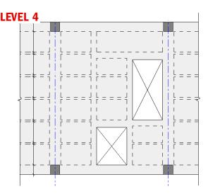
Different size pans can be used to create a void pattern that accommodates project needs. A project can use 66" wide pans as the standard void in combination with 53" and 30" filler pans to create the desired layout.
