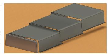
In 2013, the American Concrete Institute (ACI) introduced a way of classifying concrete for exposed conditions, but most designers still use the old classification when referring to pans; A, B, C, or D because it focuses on offsets. As Cast offsets of D (1") should be expected for projects formed using Flangeform pans with C (1/2") classifications possible with Longforms or Long-Flangeform projects. Offsets of B (1/4") or A (1/8") are not possible with pan construction.
